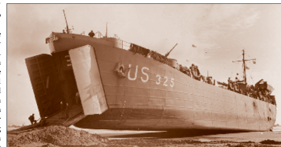
The LST, developed during World War II to carry heavy equipment and troops, could discharge its cargo directly onshore. The LST 325 became temporarily stranded at low tide on June 12, 1944, while delivering materiel to the Normandy beachhead.
